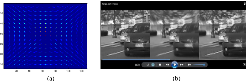
Figure 3. (a) Representation of the PSFs matrix. (b) Simulated results: an original frame (left), its corrupted version (center), the restored frame (right).
