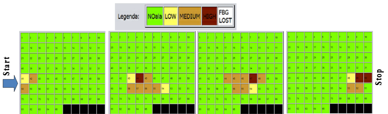
Figure 3: Intrusion Detection System software Interface: automatic detection and localization of an intrusion event
