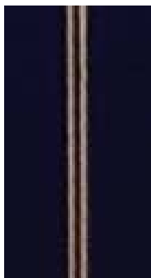
Figure 2: A polarizing microscope image of LC homeotropic alignment in PDMS channels.
