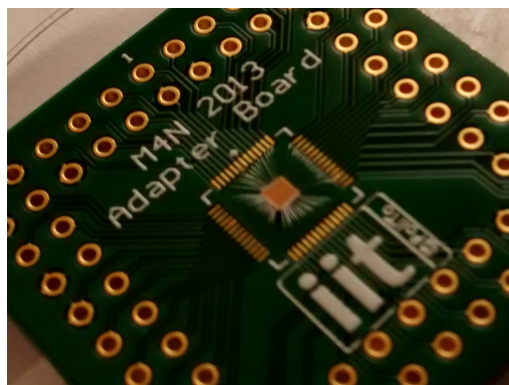
Fig. 4 : M4N prototype bonded using chip-on-board technique. The bondwires are then protected with resin before experiments.
